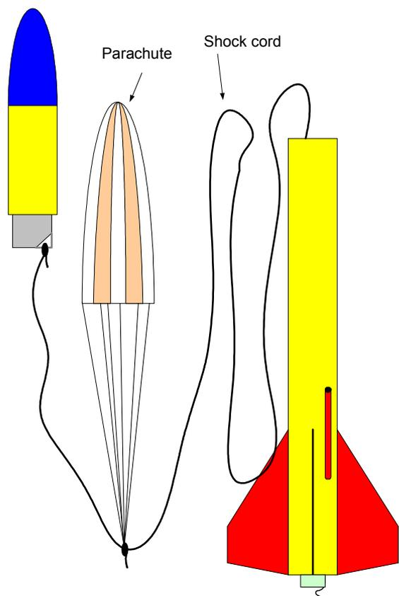
This shock cord has to be firmly attached to both the main body and the payload compartment so that it can survive the shock of parachute deployment. It is normal to make the shock cord out of a material with a bit of “give” such as elastic, but be sure to use a material that won’t melt. Some advice on shock cord materials can be found in the article “Materials for Model Rockets”.
