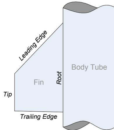
Let's start by looking at the parts of the fin. The fin is attached to the body tube at its **root**. The fore edge of the fin is called the **leading edge**, and the rear is called the **trailing edge**. The end of the fin away from the root is called the **tip**.
