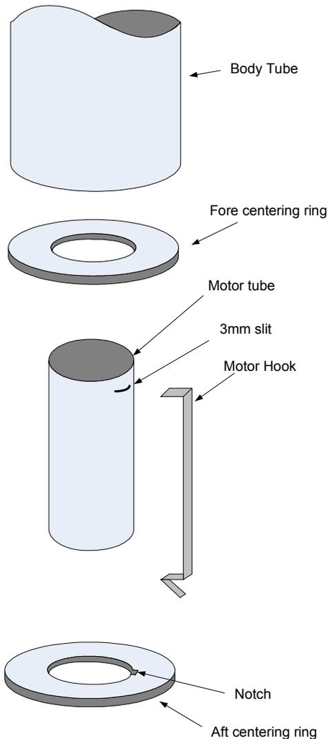
The assembly of a motor mount is quite straightforward. A diagram of the main parts is shown to the left. This includes the aft end of the body tube.
