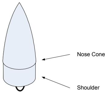
Making a payload compartment is fairly straightforward. You'll need to start with a length of body tube that is long enough to contain the payload. Allow for the length of the nosecones shoulder, as this will fit inside the tube
