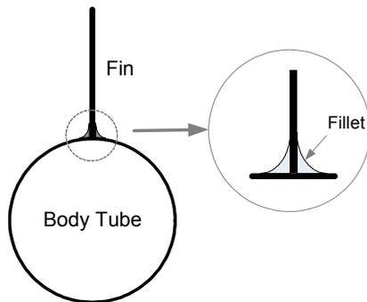
Fins can be glued directly to the body tube. This technique is called "butt mounting". It is very common in low power rockets, but is not recommended for D impulse motors of above. The basic problem with butt mounting is that the fin can tear off at higher speeds, causing the rocket to become unstable.
