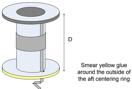
Note that this diagram is a cutaway of the body tube so you can see what's inside. Don't cut the tube open as it will severely weaken it.
