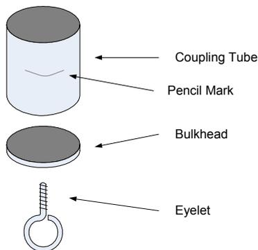
Step 4. Run a smear of glue around the inside of the aft end of the body tube. Slide the coupling tube onto the body tube up to the pencil mark and leave the glue to set.
