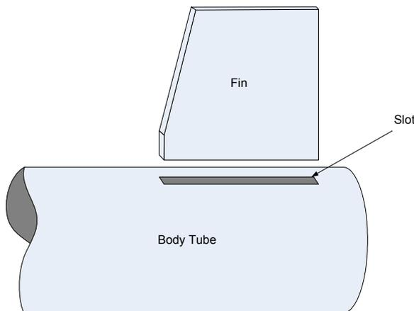
The slot needs to be the same length as the fin root, and the same width as the fin thickness. Apply some glue to the fin root and push it through until it contacts the motor tube, then apply a fillet to both sides of the fin where it enters the slot. Be very careful to ensure that the fin is straight before the glue sets.
